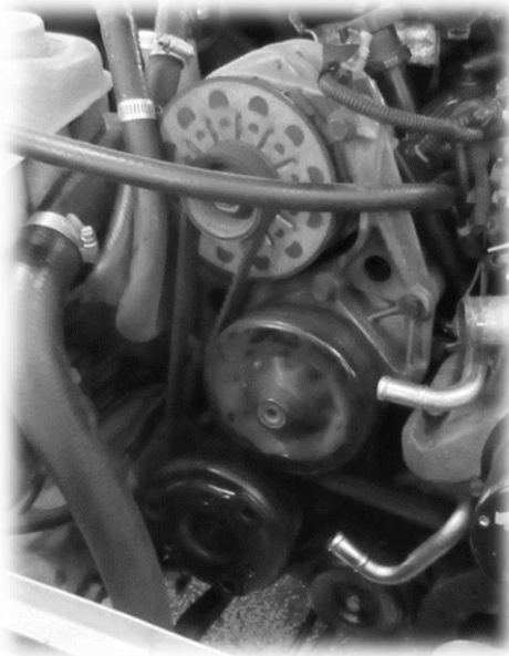
Figure 5 – Heater core hoses removed
