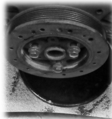
Figure 6 – Crank pulley bolts being removed
