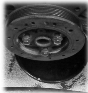
Figure 6 – Crank pulley bolts being removed
